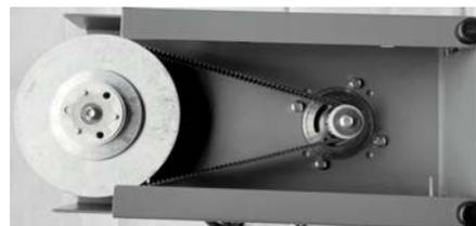
**2<sup>nd</sup> step:** Install new principal block on the motor modular and screw it.
