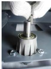
**4<sup>th</sup> step :** Install the receive pulley and screw it.
