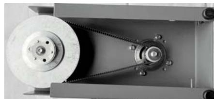
**2<sup>nd</sup> step:** Install the new belt and adjustment tightness of belt.
