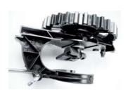
**3<sup>rd</sup> step:** Install the new QL block, you will hear "KADA", the one is at right position.
